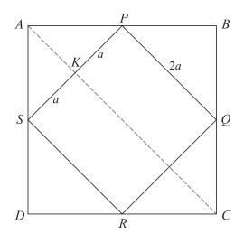
Two uniform square laminas are combined into a single body. One lamina ABCD has mass 5m and the other lamina PQRS has mass m. The lamina PQRS has side 2a, and its vertices are at the mid-points of the sides of ABCD, with P on AB and S on AD. The line PS meets AC at K, and the body rotates in a vertical plane about a horizontal axis k through K (see diagram). Find the moment of inertia of the body about k. [5]
