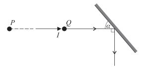
After the impact the ball Q continues in a straight line and strikes a smooth vertical barrier at an angle  $\alpha$  (see diagram). The coefficient of restitution between Q and the barrier is 0.7. Given that the direction of motion of Q is turned through 90° in the collision with the barrier, find the angle  $\alpha$ . [4]
